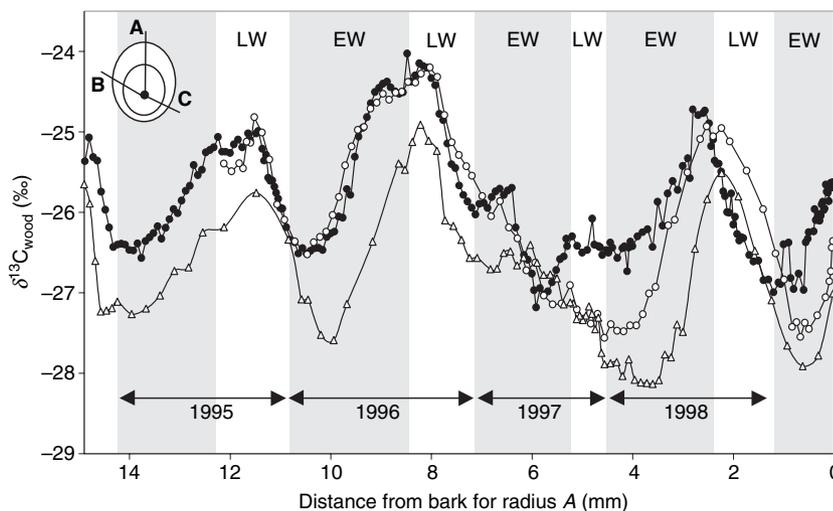
**Figure 5.** High-resolution stable carbon isotopic composition along three cross sections of stem Tw55891: A (●), B (○) and C (△). The radial section A is also shown in Figs 3 and 4. The three axes were normalized for differences in growth rates by using the visual boundaries as reference points (Section B and C were fitted to section A). Shaded background represents earlywood, white background represents latewood.
